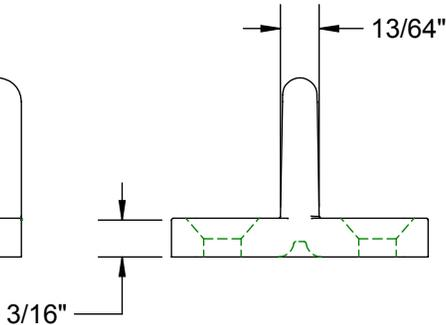
**Application:** Holds the bottom of the sliding door in place to prevent unwanted kick out. A groove needs to be routed in the bottom of the door for the guide.
