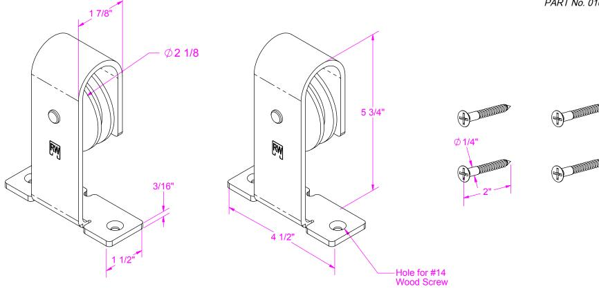
**Application:** Hangers are used on the Flat Track bar for doors 1-3/4" thick.
