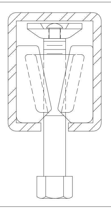
USED TO JOIN TRACK FIRMLY DURING WELDING AND INSTALLATION.
